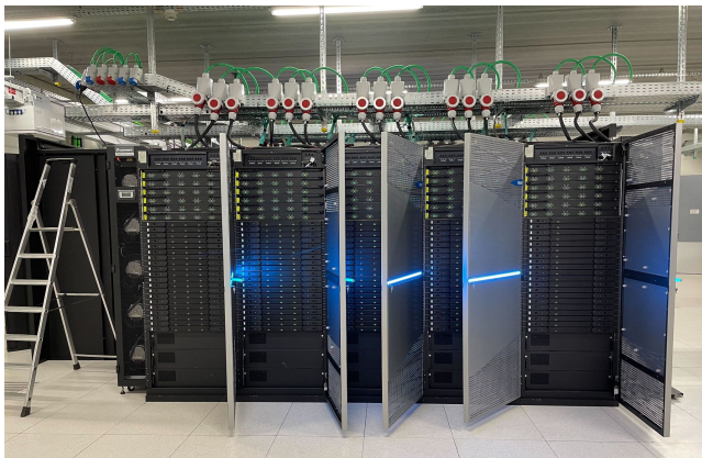
View of phase 2 of Hortense (Milan nodes + 80GB GPU nodes)
